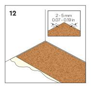
Install the underlayment directly on the adhesive, leave a space between the wall and the underlayment.
